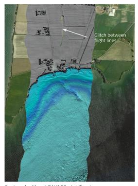
Captured without PAV100 stabilised sensor
